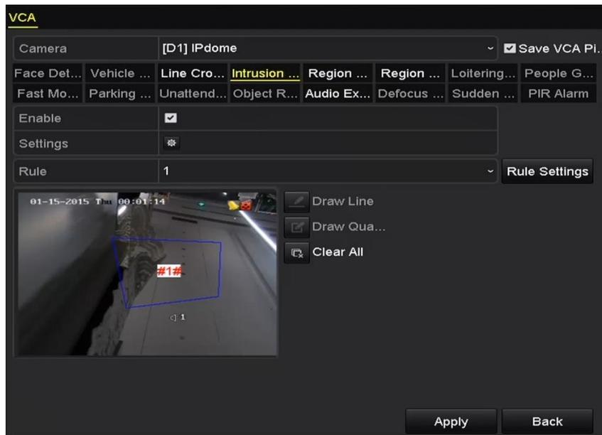
Figure 9. 8 Draw Area for Intrusion Detection
