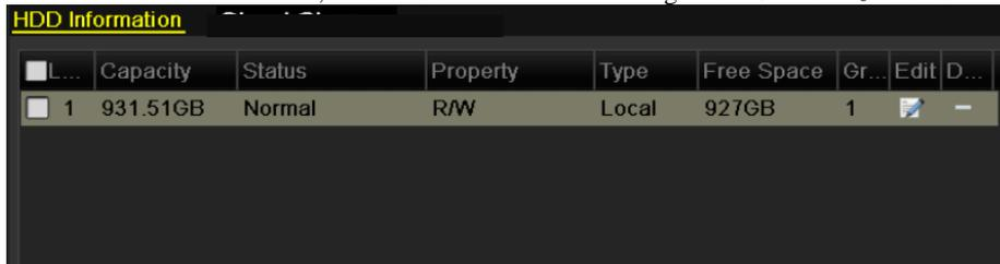
Figure 12. 4 HDD Status Changes to Normal
