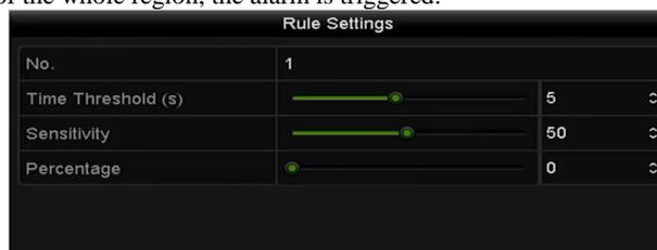
Figure 9. 7 Set Intrusion Crossing Detection Rules
